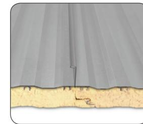
The exterior profile of the IBL roof panel has a 2"-high standing seam with the Mesa profile. The interior profile is also a Mesa pattern. The IBL panel is attached to structures with concealed clips to ensure maximum R-values.
