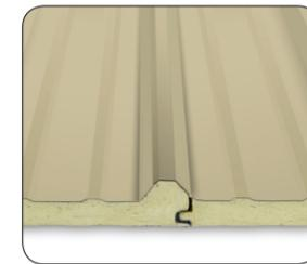
The versatility of the RWP II panel offers a multitude of design options. The RWP II can be utilized for roof or wall applications. The standard exterior skin is smooth but can be embossed if requested. The interior skin is roll-formed with our standard interior Mesa profile. The RWP II panel is the only IPS panel that utilizes a through-fastened attachment.
