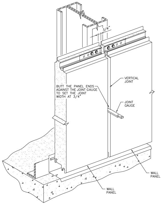
NOTES: 1. Use the 3/4" wide end of the gauge to set the joint width. Set the gauge at mid-point between the horizontal panel joints.
