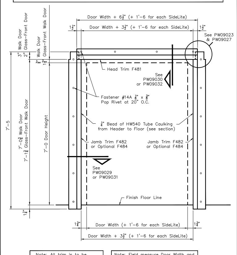
Note: All trim is to be installed BEFORE blanket insulation is applied to walls.
