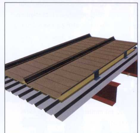
StarShield on purlins over existing metal roof.
